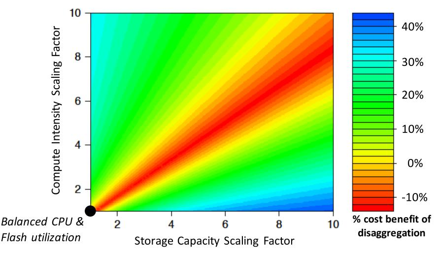
• When storage scales at higher rate than compute, save resources by deploying Flash without as much CPU
