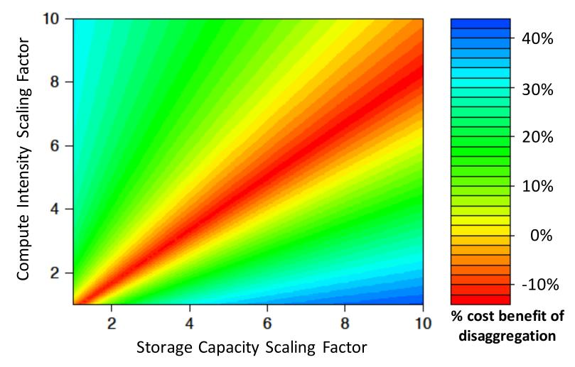
• Resource savings of disaggregated vs. local Flash architecture as app requirements scale
