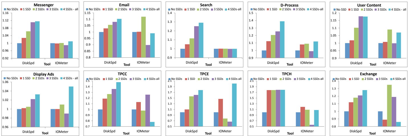
Fig. 7: IOMeter vs DiskSpd Speedup Comparison for (a) Messenger, (b) Email, (c) Search, (d) D-Process, (e) User Content (f) Display Ads (g) TPCC, (h) TPCE, (i) TPCB and (j) Exchange. The results for DiskSpd confirm the expected impact of SSD caching on workload performance. On the other hand, when the workloads are run using IOMeter there is either no performance speedup (e.g. Messenger) or inconsistent speedup (e.g. User Content) with an increasing number of SSD caches.
