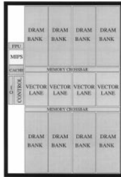
Fig. 14. Floorplan of the VIRAM-1 vector processor (drawn to scale).
