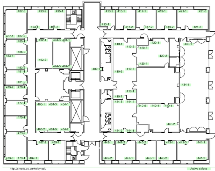
Figure 5.18. Layout of Soda Hall testbed. The code propagation experiments in Figure 5.19 injected code at mote 473-3 (the bottom left corner).
